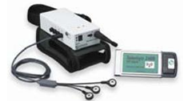
Fig. 17: Variety of EMG amplifiers ranging from 1 or 2 channel Biofeedback units to tethered and telemetric systems. Systems by NORAXON INC. USA
