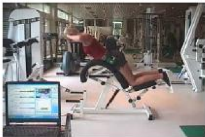
Fig. 78: Typical test arrangement and findings for static back endurance tests: Median (A), Mean Frequency (B), Zero Crossing (C) and Mean Amplitude (D), slope of a trained (green) and un-trained (blue) subject, measured for the multifidus muscle.
