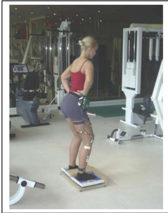
Fig.25: Cable secured with elastic straps and tape
